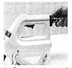
Connect water supply hose of 1/2" ID to water inlet swivel. Min. 20 PSI pressure is required for proper operation. Connect opposite end of hose to water supply. Turn water supply on.
